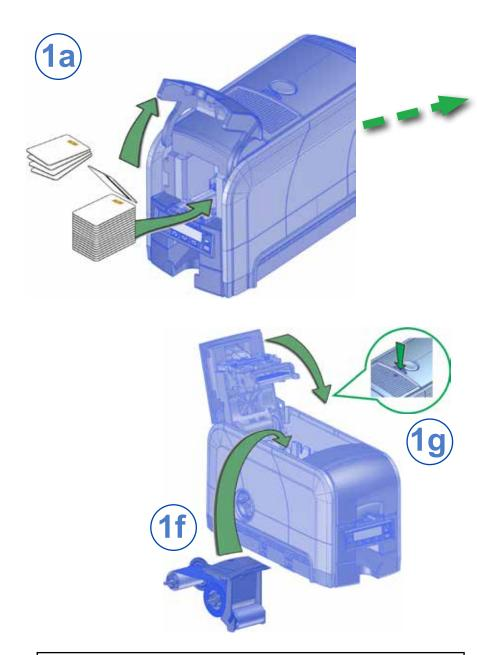
If you are setting up an SD460 system, also refer to the setup instructions shipped in the laminator carton.
